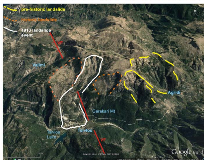
Fig. 3 a) Area affected from the 1913 Tzivlos landslide: the depletion and accumulation areas of the landslide are outlined. b) Detailed digital elevation model (DEM) of the landslide area. c) Topographic sections of the Tzivlos landslide. The sites of the sections are noted in Fig. 3a
