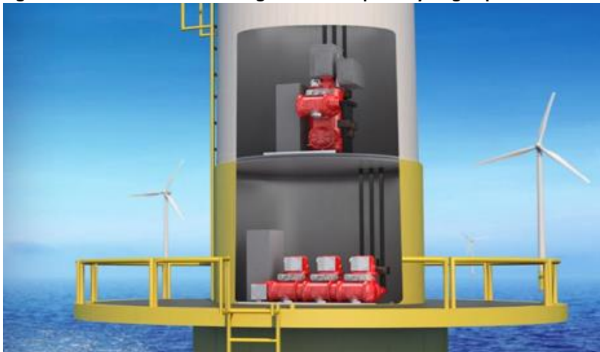
Figure 57: General Electric's integration concept of Hydrogen production unit within OWT pile
