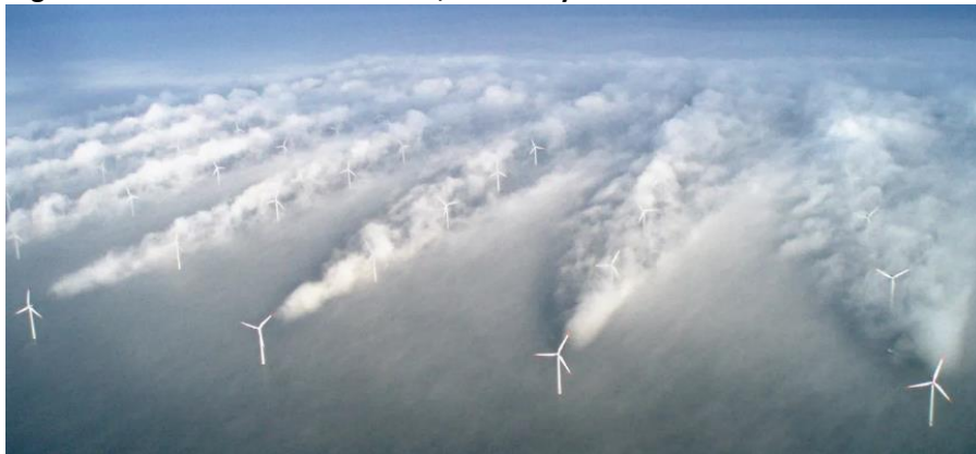
a. Wake effect in an offshore wind farm
