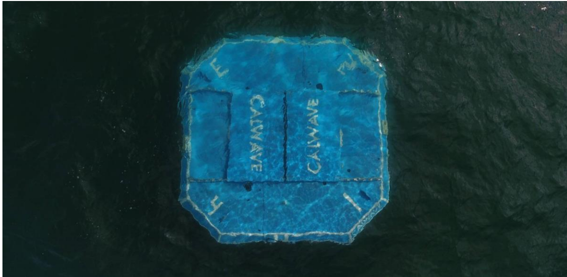
Figure 23: Submerged pressure differential WEC, which can alter its depth below water
