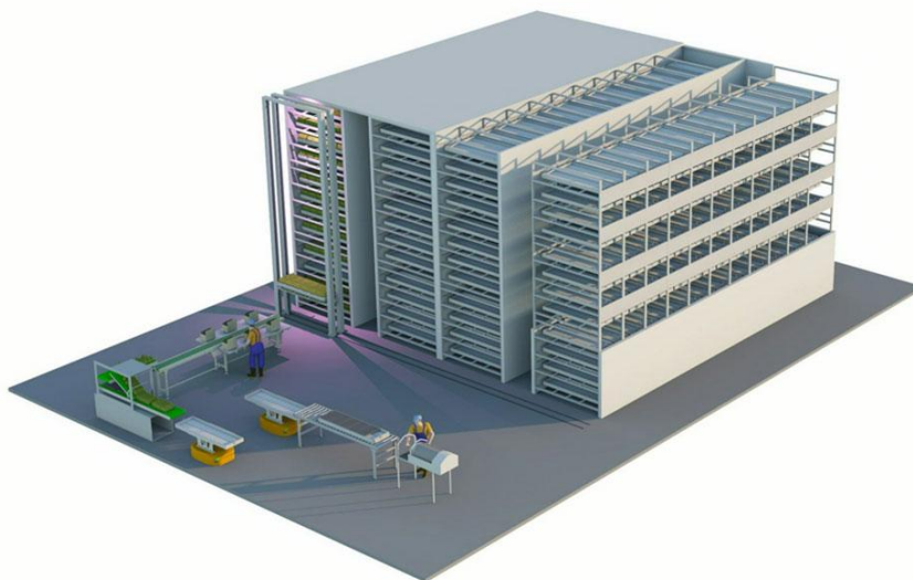
Εικόνα 16 Σύστημα Large Scale Plant Factory / Growth Solutions. https://urbancropsolutions.com/growth-solutions/ Retrieved July 16, 2024
