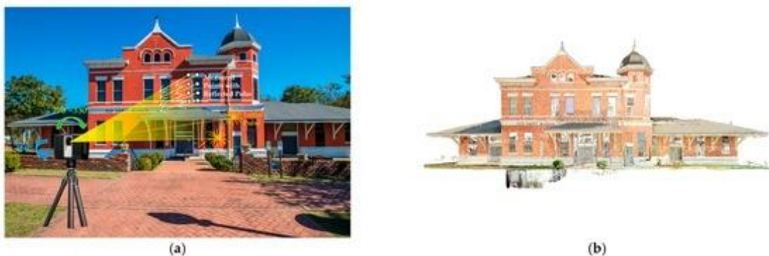
Figure 32 TLS technology and its application in heritage documentation (a) Principle of TLS. (b) A resultant point cloud of TLS survey. Source: MDPI
