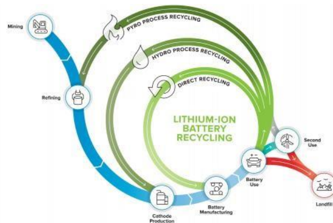
Figure G. 1: Closed loop recycling system of lithium batteries (Kunz., 2019).
