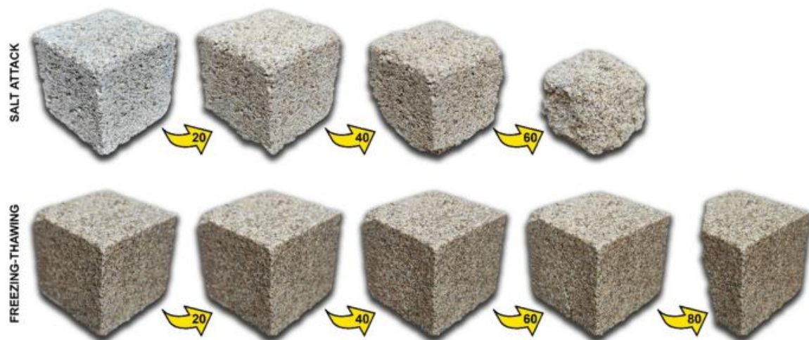
Figure 7. Heavy vulnerability of the Sfouggaria Stone against freeze-thaw action as shown in this deterioration evolution of samples after ageing tests at 20 cycle steps (Source: Coletti et al. 2025)).
