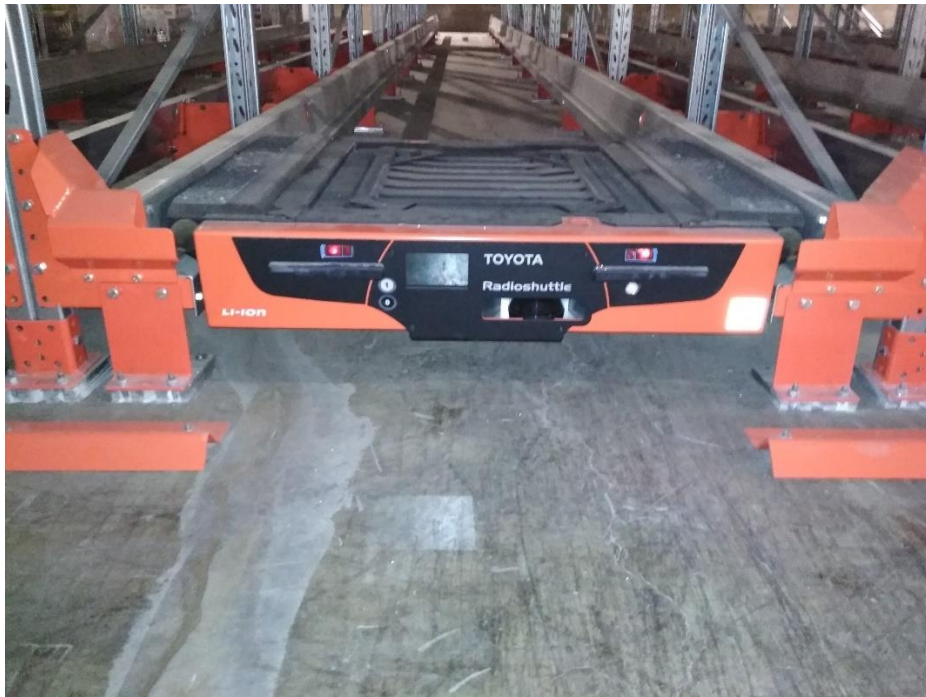
Figure 15: Shuttle of drive in racks
