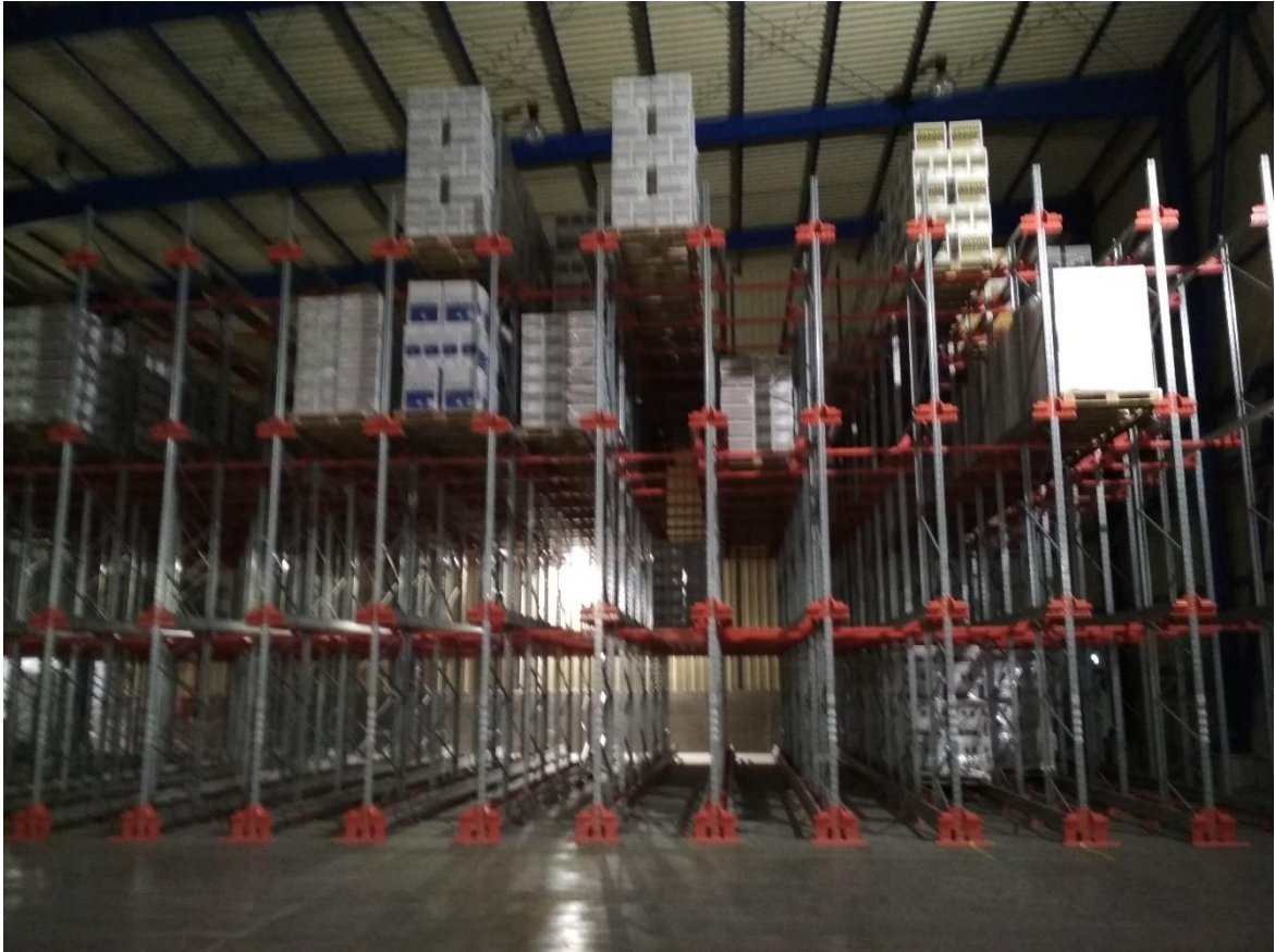
Figure 14:Finished goods warehouse: Drive In system with shuttle
