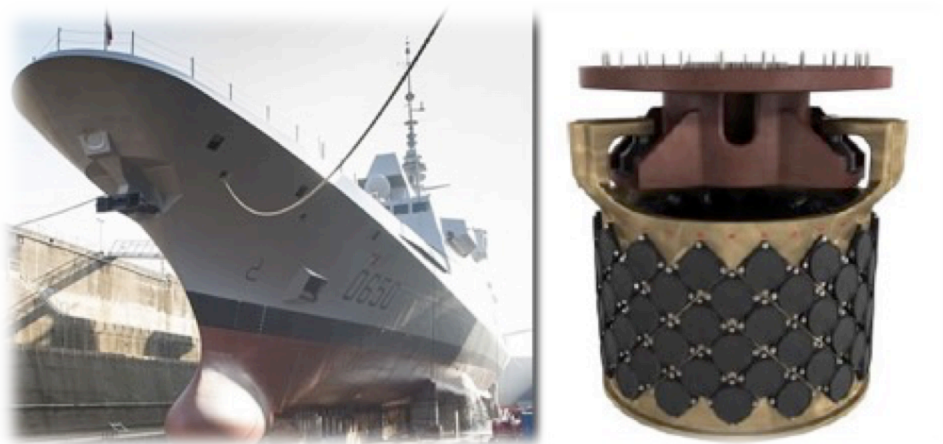
Εικόνα 35 Hull Mounted Sonar (Ανακτήθηκε την 23/5/21 από https://www.navyrecognition.com/index.php/focus-analysis/naval-technology/5504-thales-kingklip-mk2-the-next-gen-hull-mounted-sonar-of-the-french-navy-fti-frigates.html )
