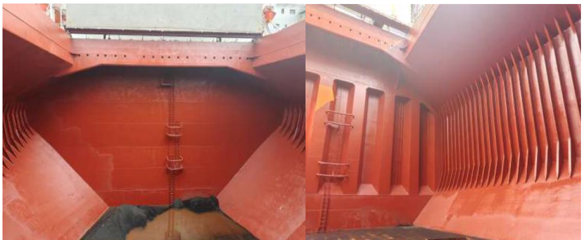
Figure 17 Apply 2nd coat in cargo holds
