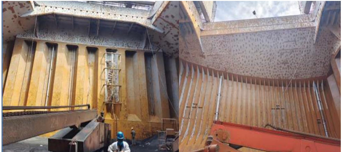
Figure 16 After HPFWW in cargo holds
