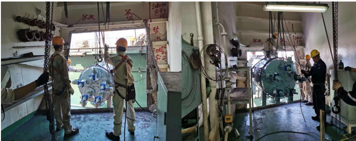
Figure 20 BWTS filter shifting
